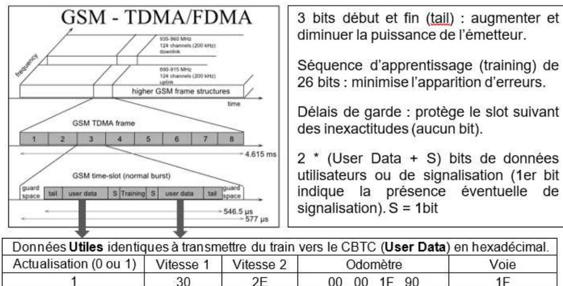
Figure II-3 : TDMA – (*time division multiple access*).
